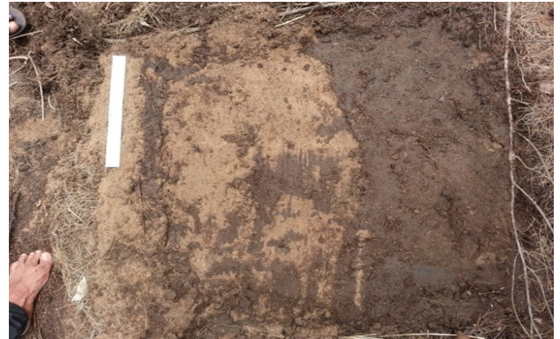
Figure 8: Selective penetration of water into the soil causing irregular wetting patterns
